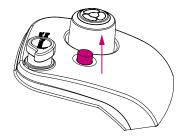
**Pressurized** The float valve has visibly popped up above the surface of the lid.
