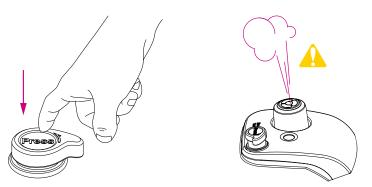
When depressed, a stream of steam releases through the top of the steam release valve.
