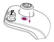
**Depressurized** The float valve has descended and the top is flush with the lid.
