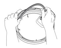
With the sealing ring removed, check the ring rack to make sure it is secured, centered, and an even height all the way around the lid. Do not attempt to repair a deformed ring rack.
