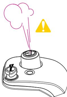
When depressed, a stream of steam releases through the top of the steam release valve.
